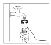
**2.** The other end of the inlet hose which connects to the machine can be turned as showed in the picture.
